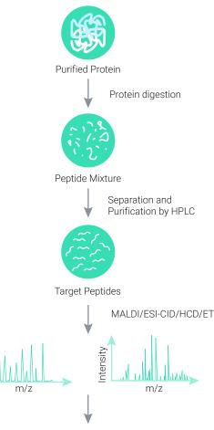
Using the de novo sequencing analysis software to analyze the peak map of specific fragmentation ions to obtain the mass of amino acids
